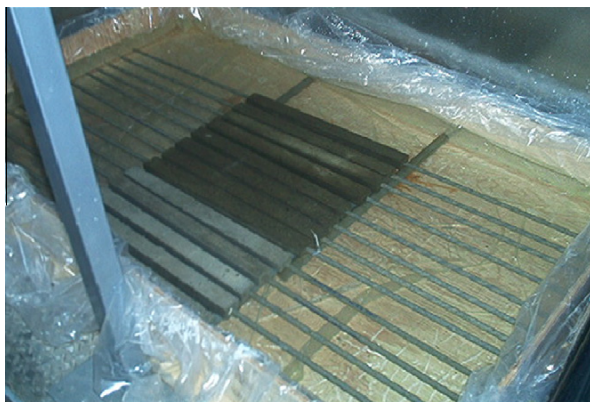
Fig. 2. Wood container built for aging of the cement mortar-wrapped GFRP bar specimens.
