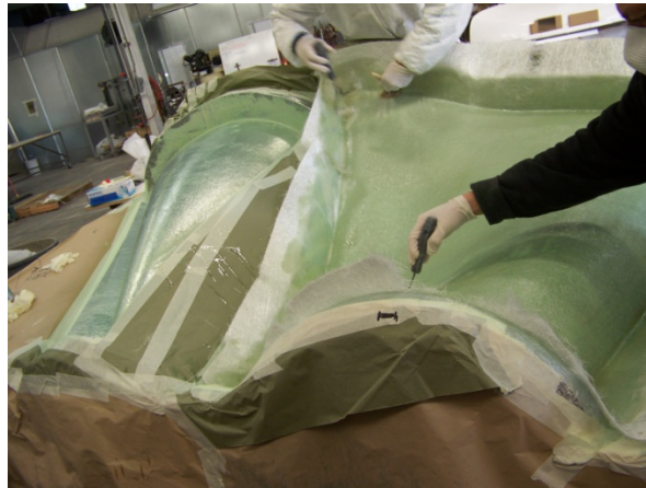
Hand layup of FRP on an open mold
